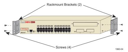
Figure 3-3 Installing the Rackmount Brackets
